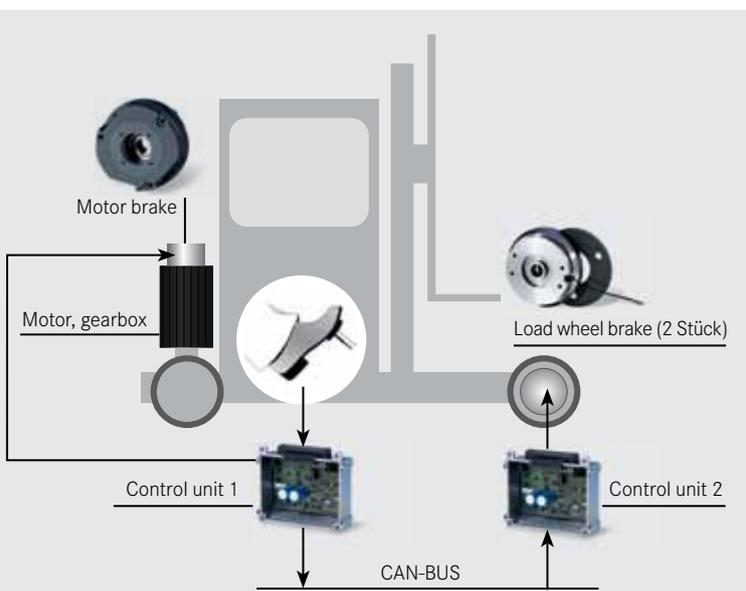
Example of a completely controlled brake system
