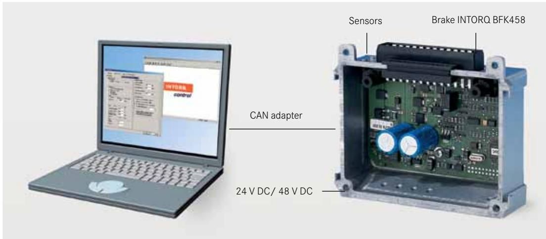
The mechatronic brake system is suited for controlled braking in battery-driven stacker vehicles. The combination of a spring-applied brake with an intelligent control provides an optimal load-dependent braking torque control (load-independent stopping distance). The control range covers 20 % to 100 % of the rated torque. The parameterisation of the INTORQ Control is done via the Windows user interface.
